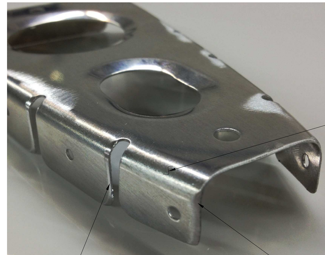
FIGURE 2: RIB FLANGE PREP
