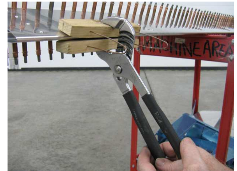
FIGURE 5: TRAILING EDGE TOOL APPLICATION
