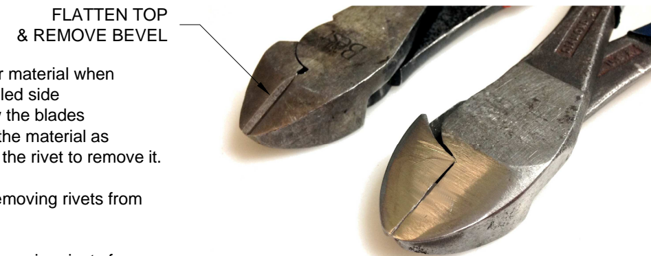
FIGURE 3: MODIFY SIDE CUTTERS
