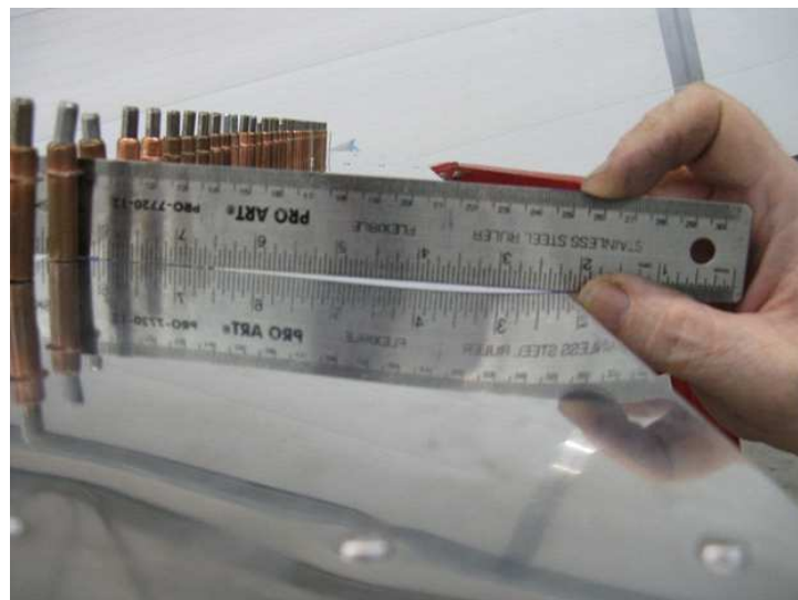
FIGURE 3: OVER BENT TRAILING EDGE
