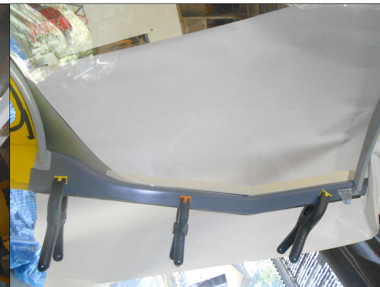
FIGURE 2: MOLDING CLAMPED IN PLACE
