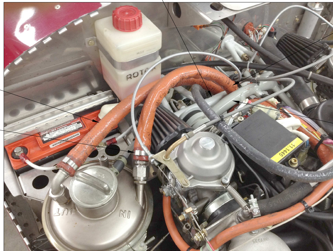
FIGURE 2: INSTALLING THE OIL HOSES VIEW FROM ABOVE
