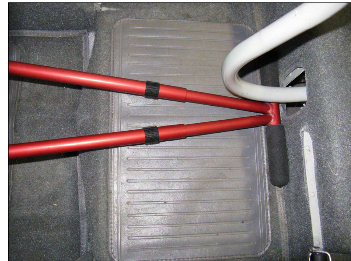
FIGURE 3: CONTROL LOCK POSITION AGAINST BULKHEAD
