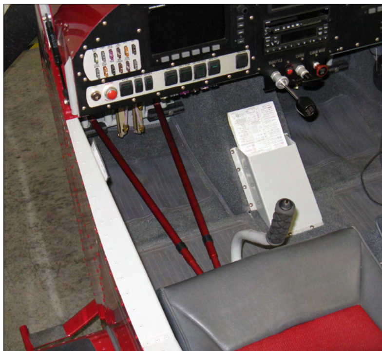
FIGURE 1: CONTROL LOCK INSTALLATION OVERALL VIEW
