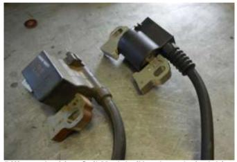
Figure 9 - Different Ignition Coil Models (Honda on Left, Jabiru on Right).
