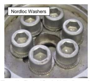
Figure 10 - Flywheel fitted with Nordloc washers
