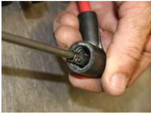
Figure 6 - Adjusting High Tension Lead Caps
