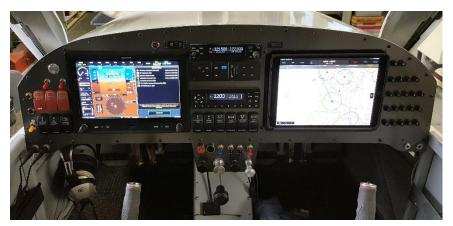
1 0 GTR 200 COMM GMC 305 AUTO PILOT (ii) (ii) GARMIN G3X TOUCH IPAD with GARMIN PILOT 5050  $\hat{\underline{\Phi}}^{*}\hat{\underline{\Phi}}$ GTX 345 w ADSB TRANSPONDER 50000 ----۲ 0000 UKUDK UKU KUBU 00000 .... 0 0 00 • <u>•</u> <u>•</u> <u>•</u> <u>•</u> © (P8) CH)
