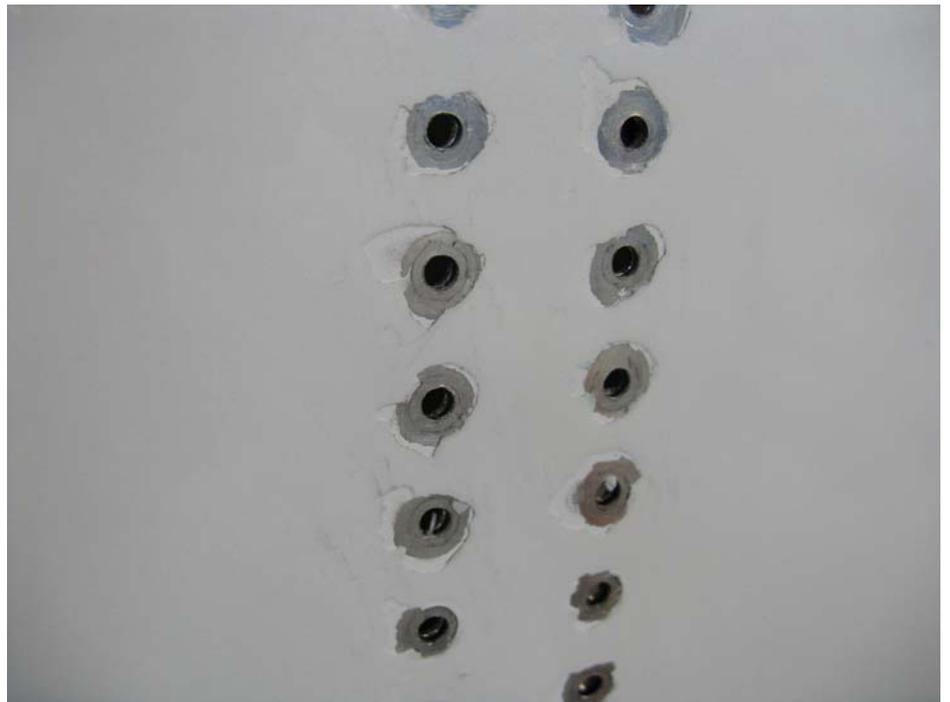
**FIGURE 8:** REMOVED RIVET
